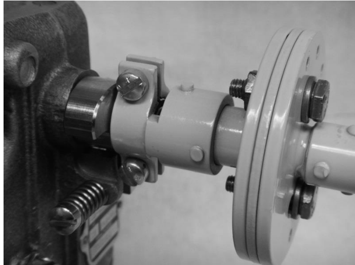
Figure 5-10b: Proper Positioning of Carburetor Stop Arm and Throttle Linkage Adaptor
