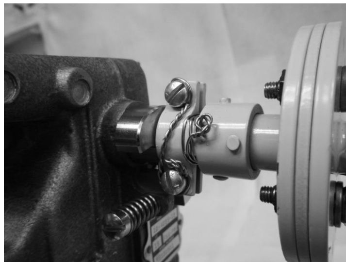
Figure 5-10e: Securing Throttle Linkage Adapter to Carburetor Stop Arm with Safety Wire
